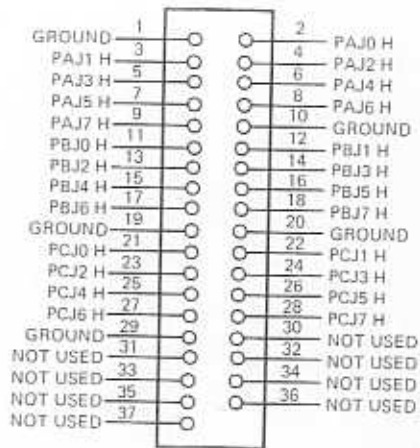
Figure 20 Pin Signals on 37-Pin Parallel I/O Connector (BCC12 Cable Only)
